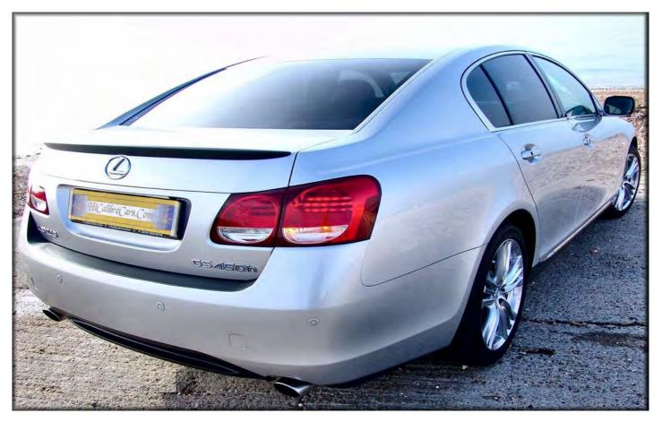
Subaru Impreza territory. At slow speeds the GS will run silently on its electric motors, while at moderate or cruising speeds, the petrol engine drives the wheels and recharges the battery. At full chat, the Lexus is powered by both its 292bhp 3.5-litre V6 engine and electric motor. Combined power adds up to the equivalent of a 450bhp V8 (hence the GS 450h badge).
